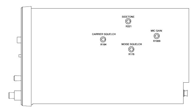
FIGURE 2-1 KY 96A, KY 97A Cover-On Adjustments
