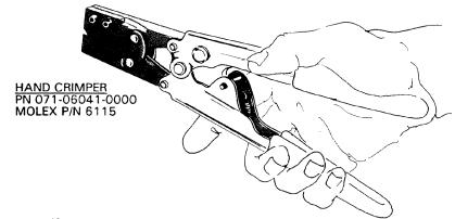
Close crimpers until ratchet begins to engage. Then insert the terminal into the jaws from the back side. (See Figures at bottom of page) For 24 to 30AWG wire, it will be necessary to start the crimp in jaw A and then complete it in jaw B.
