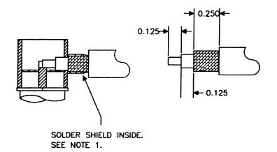
RG-400 P/N 024-00051-0060 USED ON NAV, COM, DME, XPONDER AND RADIOTELEPHONE.
