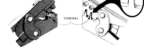
Terminal is in correct position when insulation tabs are flush with outside face of crimp jaws.
