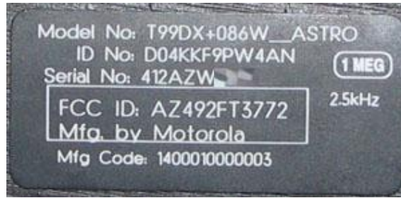
Figure 5.2 A photo illustration of a model number tag on the rear of a Motorola Inc. ASTRO Digital Spectra™. There are several useful pieces of information displayed in the tag, including the model number, serial number, manufacture code (FLASHport™), host firmware flash ROM size (1M) and indication of a 2.5 KHz narrow-band RF board.
