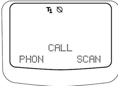
Figure 6.3 Motorola Inc. XTS 5000™ screen display when Type 1 encryption algorithm is in use. Note the T1 indicator.
