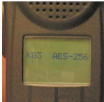
Figure 11.6 Contrary to incorrect information posted on a certain Internet discussion forum, the ASTRO™ products do support the AES-256 Type 3 encryption algorithm. Featured in the photo illustration is an XTS 3000™ with a DES-OFB/DES-XL/AES-256 triple-algorithm UCM module installed. This algorithm is also referenced in both the ASTRO™ portable and mobile host ROS firmware builds.
