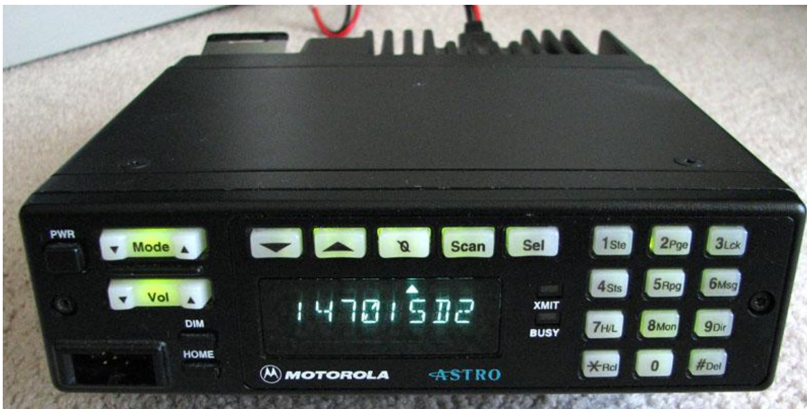
Figure 5.1 A photo illustration of a Motorola Inc. ASTRO Digital Spectra™ in a W7 dash-mount configuration. Pictured is the 50W version.
